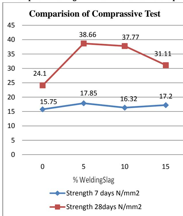
Fig2. Relation between compressive strength of M25 concrete at various percentage of Welding slag.
