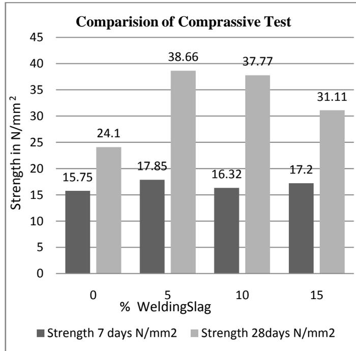
Fig1. Relation between compressive strength of M25 concrete at various percentage of steel slag.
