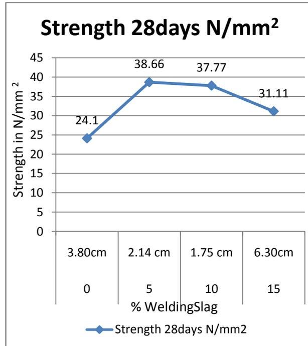
**Fig 4. Relation between compressive strength and Carbonation depth of M 25 concrete at various percentage of Welding slag.**
