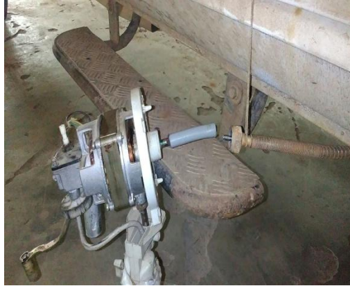
Fig 1 Attaching the Odometer cable to the fan.
