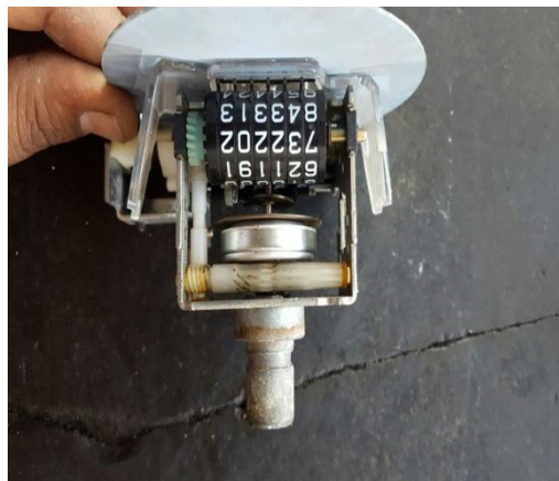
Fig 5 Gear train of Odometer for adjustment
