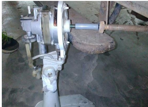
Fig 2 Running of fan increasing odometer reading.
