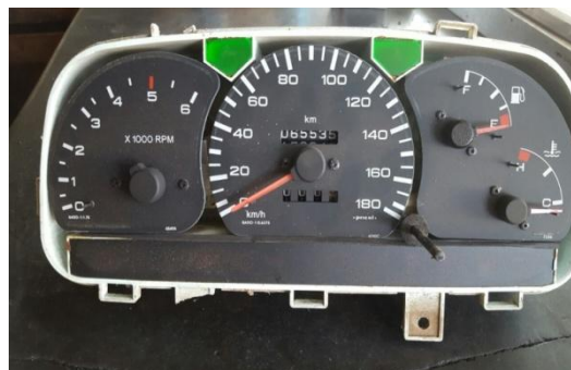
Fig 3 Front view of Mechanical Dash Board
