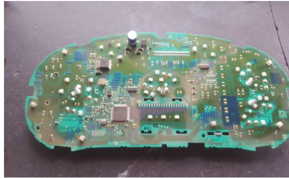
Fig 11 Top side of internal digital dashboard
