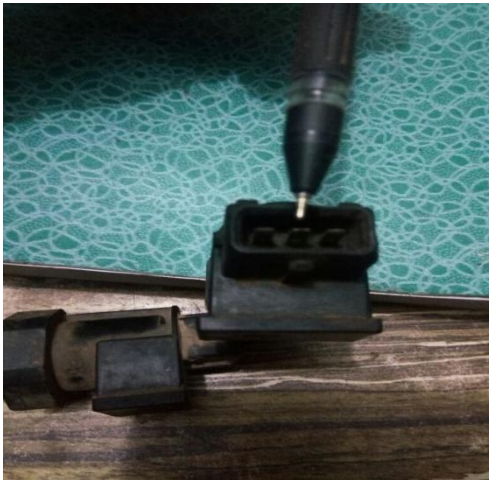
Fig 8 Tapping of wire for increasing odometer reading
