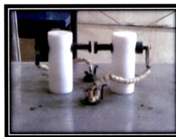
Fig.2.3. Sample holder for the conductivity measurement.
